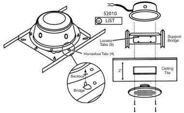
Compound knockouts provided for metallic UL Listed fittings for  $\frac{1}{2}$ " and  $\frac{3}{4}$ " plenum rated cable and plenum whip flex conduit.
