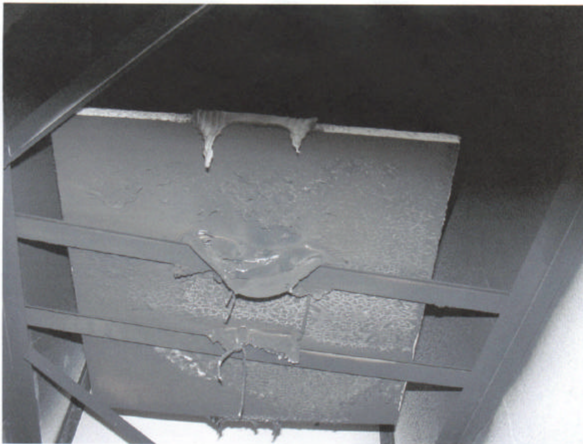
Photograph 12 – Bottom view of speaker assembly after to burn 020326b
