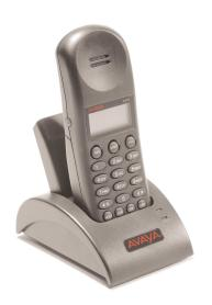
Only NiMH Battery Packs with a YELLOW label on the handset contact side may be charged in the Dual Battery Charger. Nickel-Cadmium (NiCd) and older NiMH Battery Packs with a GREEN label will not charge. If the indicator light does not come on when a Wireless Telephone or Battery Pack is first placed in the Charger, check to make sure the Battery Pack has a YELLOW label.
