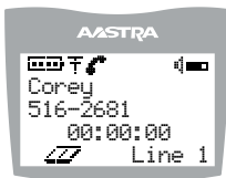
Private Call in Progress
